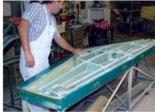
Horizontaal stabilo in wording. (Foto: Diamond Aircraft)
