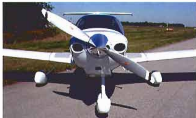
LEFT: Pick your prop. This aircraft has the Hartzell two-blade constant speed propeller, but the three-blade MT composite prop is still an option. RIGHT: The wing section is a modified WORTMAN FX 63-137/20 laminar airfoil specifically designed for this aircraft. The wing design, with upturned wingtips, provides for benign stall characteristics.
