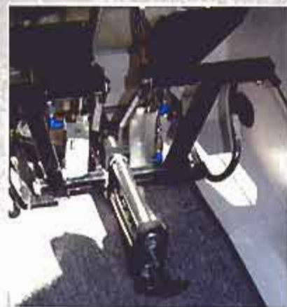
The rudder pedals come to you. Because the seats were crash tested to -26Gs as set, designers had to build the rest of the pilot's position around them.
