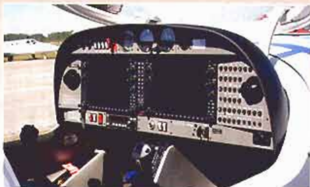
LEFT: Entry is easy for both pilots and passengers alike. RIGHT: The inside of the plane looks as modern as the outside—the Garmin G1000 panel is now one of three options for avionics that Diamond buyers have.
