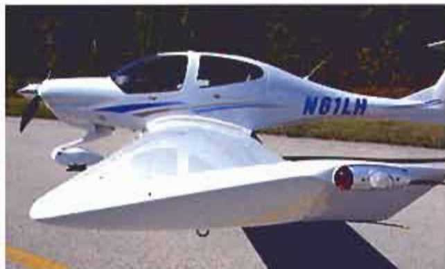
LEFT: Pick your prop. This aircraft has the Hartzell two-blade constant speed propeller, but the three-blade MT composite prop is still an option. RIGHT: The wing section is a modified WORTMAN FX 63-137/20 laminar airfoil specifically designed for this aircraft. The wing design, with upturned wingtips, provides for benign stall characteristics.
