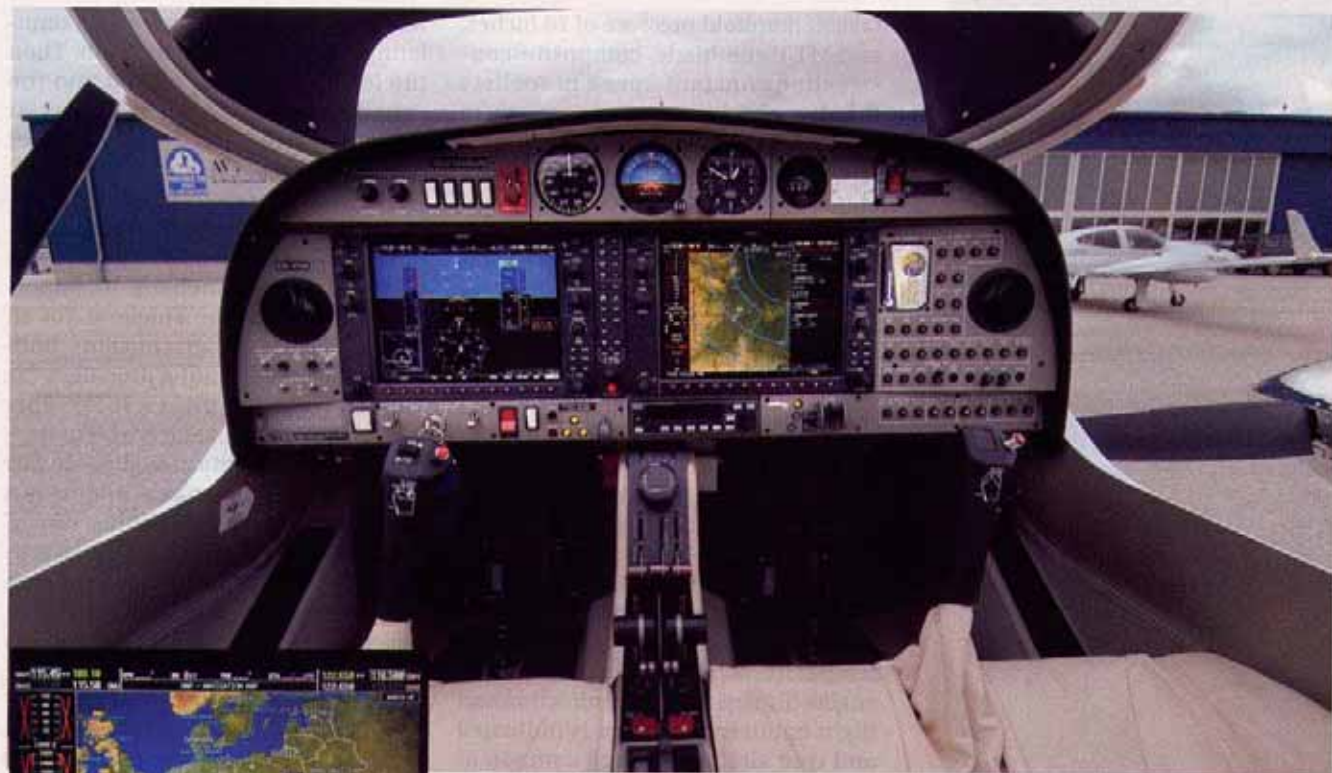
The avionics package features a two-display Garmin G1000. Its multifunction display can be zoomed in or out (left) to show a massive moving map. Diamond's Austrian factory is in the dead center of the screen. For now, a Bendix/King KAP 140 serves as autopilot; a Garmin unit will soon replace it.
