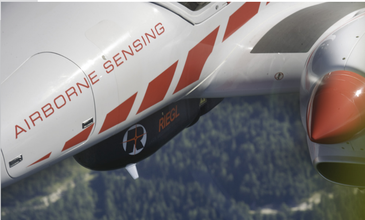
DA42 Multi-Purpose Platform laser scanning mission
