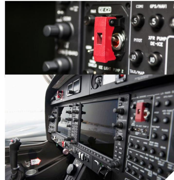
A proven TKS ice protection system helps the DA42-VI to withstand flight into known icing conditions. Wings, tail, propellers and windshield are protected with TKS fluid, systems are redundant and rigorous flight tests have demonstrated the ability of the DA42-VI to withstand icing long enough to get you back to safety.
